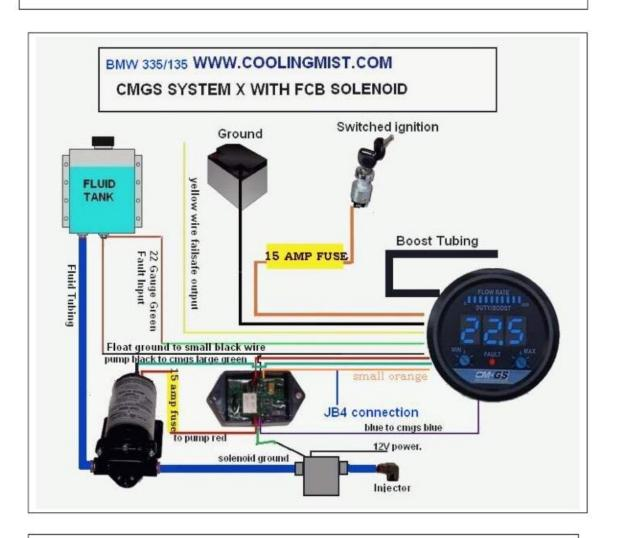
When setting up the CMGS System X for the JB4 the small orange FSB wire connects to both the small CMGS orange wire and PIN #15 on the DSUB for the JB4.
